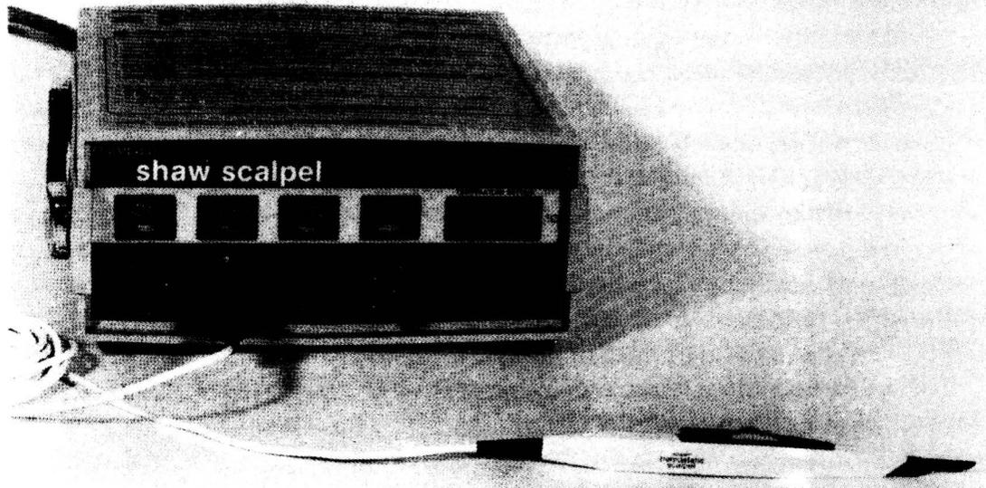
**Fig. 1.** The Shaw haemostatic scalpel. The controller unit and the handle with the blade
